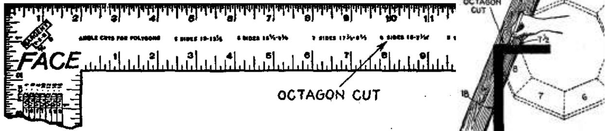
Suppose we want to create an n-gon where n is at least 5. The polygon table is constructed by finding rational numbers a and b with denominators equaling 8 so that  $\tan \frac{\pi}{n} \approx \frac{a}{b}$ :
