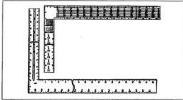
Using the tables and scales that appear on the blade and the tongue is a vanishing art because of computer software, construction calculators, and the availability of inexpensive prefabricated trusses.
