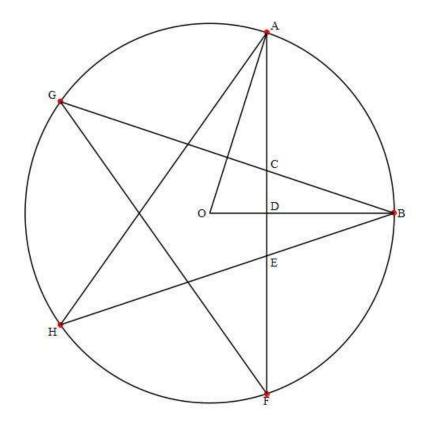
Here O is the center of the circle. We have drawn lines from O to two vertices of the star, A and B. Points C and E are where BG and BH intersect AF, respectively, and D is where OB intersects AF. Note that triangle CEB is a *golden triangle*, an isosceles triangle with apex angle 36 and base angles 72 degrees. Let us call the lengths of line segments |CB| and |CE| a and b, respectively. Then, because triangle CEB is golden, we have:
