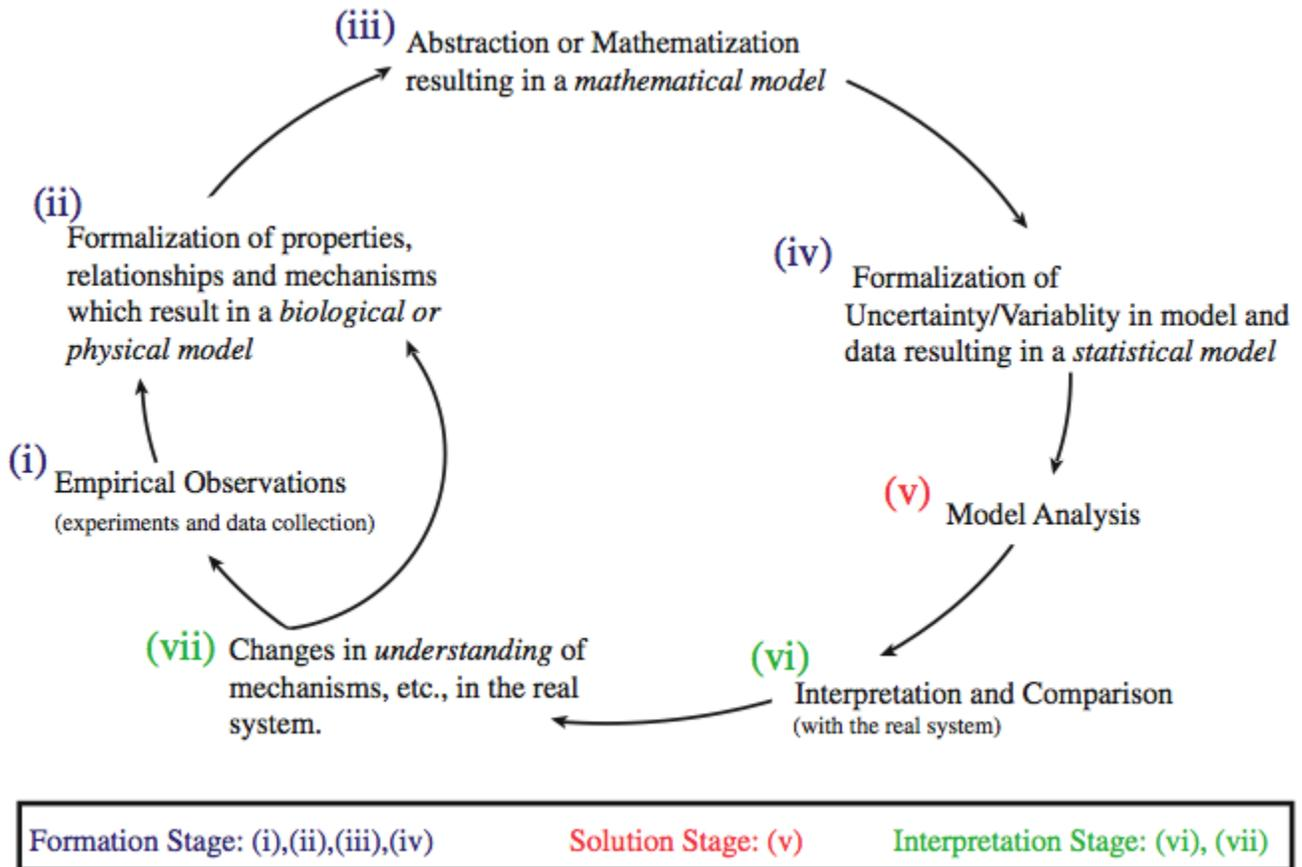
Figure 3.1: The Iterative Modeling Process [3].
